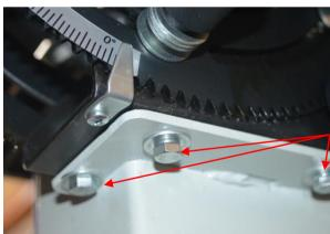
This pointer is adjustable if the setscrew is loosened. You may need to make a small adjustment after the table is set perpendicular to the blade.
