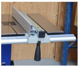
The rip fence is reversible and may be used on either side of the blade.
