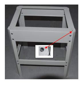
Carefully align the parts until the stand is square and ensure that the 4 large holes in the top corners are lined up as you will need to put bolts through these to fix the saw to the base.
