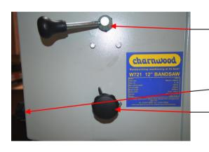
Quick blade tensioner (shown in tight position). Looking from the front of saw, turn the lever anticlockwise to slacken the tension.
