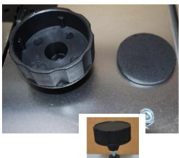
Locate the tension adjustment knob and using a suitable tool, remove the cap. Be careful not to lose the nut which is inside.
