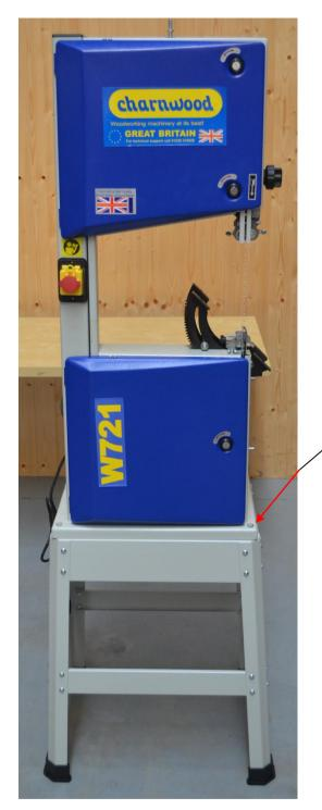
If you have someone to help you, the easiest way to join the saw and the stand is to lift the saw and lower it into place. Secure it with the four countersunk setscrews, washers and nuts provided.
