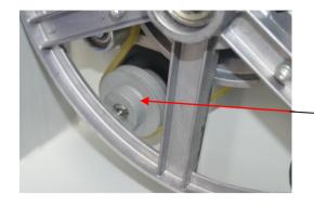
Release the belt tension by turning the tension control handle on the front of the lower housing. Move the belt from the larger pulley to the smaller one and then from the smaller to the larger on the other pair. Always have the drive belt on one large and one small pulley.
