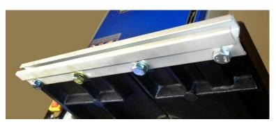
Attach the Rip Fence Carrier to the front edge of the table using the four M8 x 12mm bolts provided.
