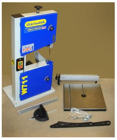
After cutting the tape at the top of the box, invert it on a table or bench and lift it off the polystyrene insert. Separate the two pieces of packing and remove all the components.
