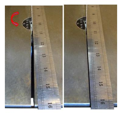
Twist the table on the trunnion until the rule is aligned with the slot.
