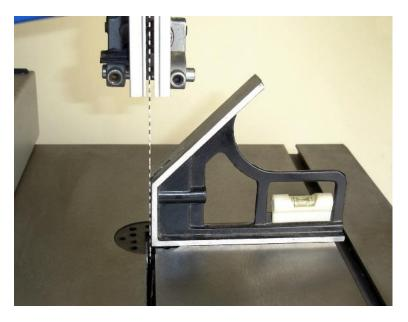
Having set the table so that the blade is centred, use a set square position the table at right angles to the blade.
