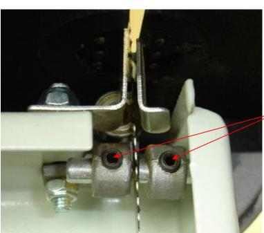
Slacken the guide pin locking screws then adjust the pins so that there is a clearance of 0.5mm either side of the blade. Lock the pins in place with the grub screws.
