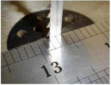
Carefully place a steel rule against the side of the blade, between teeth.
