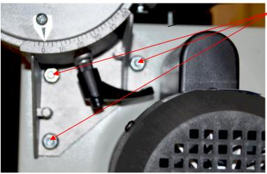
The lower trunnion is attached to the body of the saw by three hex headed bolts.
