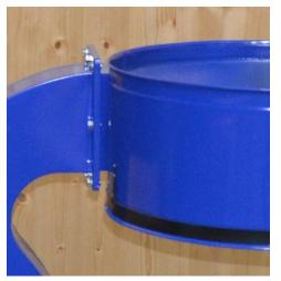
Offer up one of the collector bodies (please note: the left and right side are different). If this is done carefully, it will be possible to engage each of the bolts with the thread which is tapped into the flange of the collector body. Leave them loose until all are engaged, then tighten them securely.
