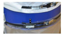
Now fit a bag clamp around the outside of the bag to secure it.
