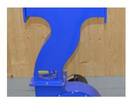
Place the Y shaped outlet over the gasket as shown and fix it to the flange using 8 of the M8 x 16mm bolts, washers and nuts.
