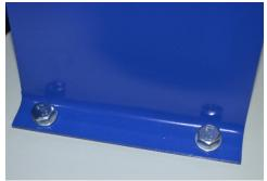
Turn the base so that it is standing on its castors and bolt on the motor support bracket. Use 4 of the M8 x 16mm hex headed bolts and washers.
