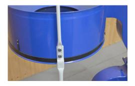
Now attach the upper end of the collector support and the upper bag support to the collector body.
