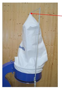
Using the small loop located at the top, hang the filter bag on the bag support and gently stretch the bottom of the bag over the rim of the collector body.
