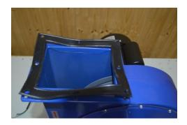
Place the rubber gasket on top of the air outlet.
