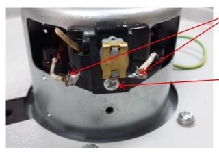
The 2 remaining copper wire connections to the brush are clamped in place by a folded tang. Unfold the tang to release the wires.
