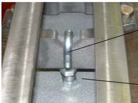
Fig 3: Sketch showing assembly of additional J-bolt clamping on the web.
